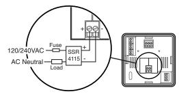
Figure 3.11 Control Output Wiring–DC
